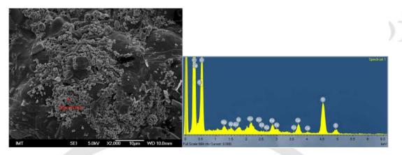
Fig. 2. (a) Nano-TiO<sub>2</sub> dispersed over the lower leaf surface to give a final concentration of  $5,000 \mu g/g$  dry weight leaf. The red spot indicates where the spectrum for energy-dispersive X-ray spectroscopy analysis was performed (EDS) (b), to confirm the presence of Ti.
