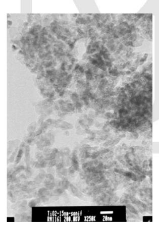
Fig. 4. Transmission electron microscopy of tested nanosized  $TiO_2$  particles, showing their shape and size.
